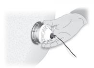
Unscrew light socket plastic support and remove light bulb or CLS-2.
